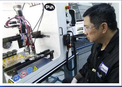
Conformal coating of optoelectronic subassembly
