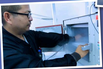
Thermal shock and cycling: 100% production part environmental inspection and test, with simultaneous signal integrity qualification
