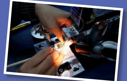
Final assembly, PCB-mount optoelectronic transceiver
