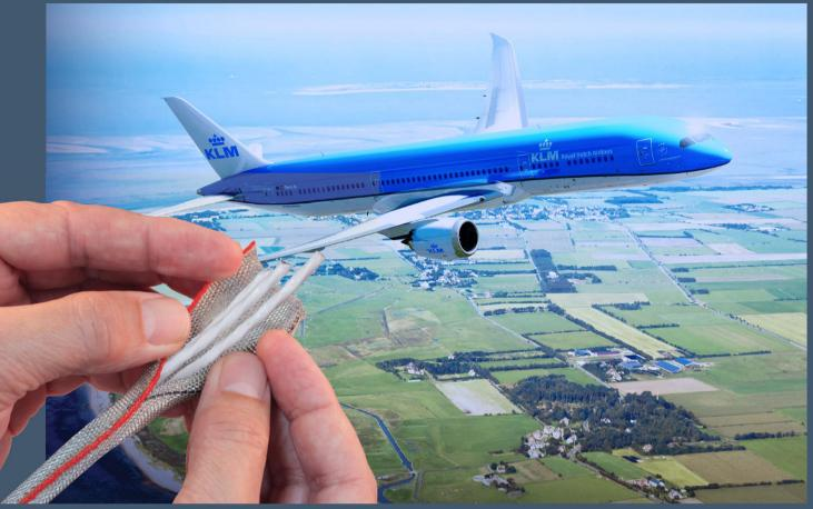
Tubular braided sleeving meets the broad range of EMC shielding and mechanical protection requirements of aircraft harness assemblies. But the need to apply shielding materials over already-installed aircraft wire and cable bundles requires new technology. Legacy self-wrapping cable braid has long been available for EMI/RFI applications and abrasion protection, albeit with poor performance due to its heavy weight, inflexibility, and "windowing," which results in poor shielding performance.
