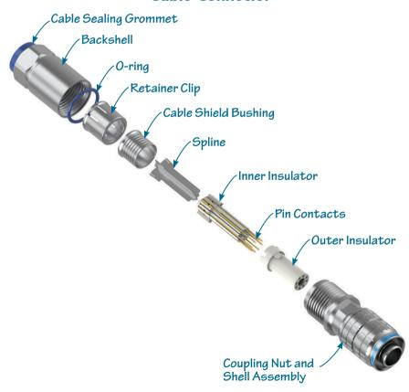
Cable connectors feature gold-plated crimp contacts, precision insulators, integral backshell, sealing grommet and machined shells. Cable connectors are available as unassembled kits or ready-to-use factory-terminated cordsets.
