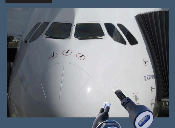
Environmentally-sealed breakaway design for high-speed data transfer between terminal gate and aircraft
