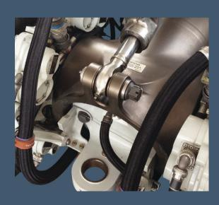
Turnkey wheel well impact-resistant metal-core conduit assembly
