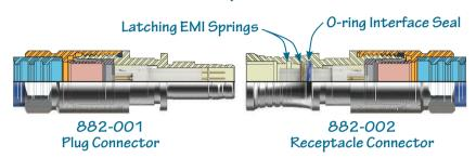
Push-pull SuperFly Datalink receptacle connectors feature two canted coil springs for secure mating and excellent EMI protection. A fluorosilicone O-ring provides watertight sealing when mated.
