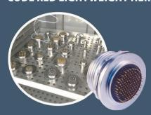
Connectors utilizing CODE RED hermetic encapsulant sealing underwent a grueling qualification test and validation process to prove material durability and hermeticity. Validation testing including 100 cycles of thermal shock IAW EIA-364-32 Test Condition A -65°C to +200°C while maintaining hermeticity followed by 1000 hours of thermal aging at 200°C. Additional tests included:
