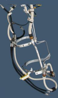
Metal-core conduit wire protection aircraft brake assembly
