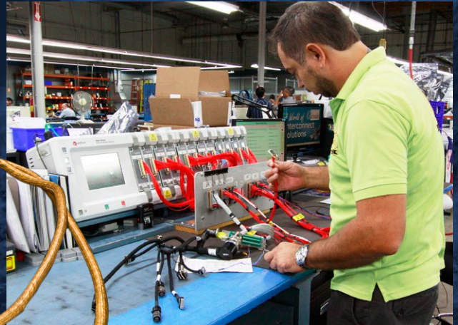
Continuity testing standard on all cable circuits
