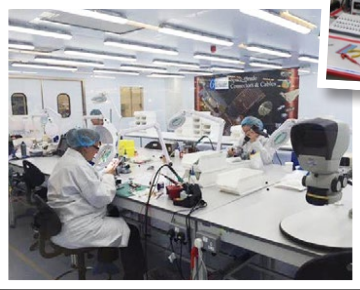
The Glenair Mansfield clean room assembly area is used for fabrication of laser, space, and satellite assemblies IAW ISO Class 8 -100,000 PPM
