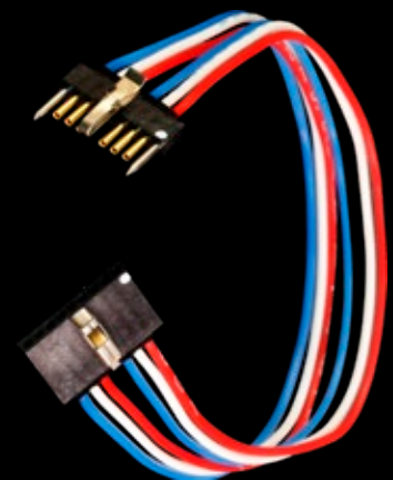
.050" pitch single row surface mount back-to-back microstrip
