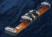
Space-grade Micro-D flex assemby with NASA EEE-INST-002 screening
