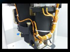
Harness integration into space payload electromechanical devices
