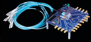
Available evaluation boards: 050-346 parallel optic transceiver with MT-to-39029 fiber optic terminations
