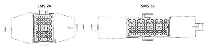
Contact identifications shown are for mating face. Contact identifications of wiring face are identical as shown on the receptacle arrangements
