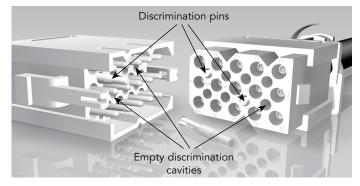
A pin, which can be inserted in the discrimination cavities of the SMS Quick mating cable and boardmount connectors. The discrimination cavities are in between of the contact cavities and offer the advantage that no contact cavities are lost due to discrimination.
