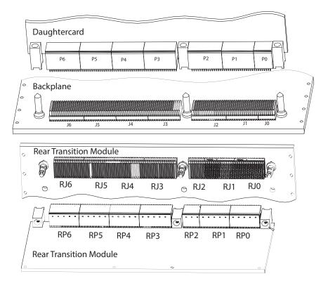
Note: RT 2 or RT 2-R PO connector can be used assuming wafers 7 and 8 (dff pairs) do not require higher data rates. These connectors have smaller compliant pins in columns 7 and 8 and RT 2 compliant pins in columns 1-6 (mixed hole pattern). RT 3 PD BS J0 (2332816-18 2332817-1) have smaller compliant pins in columns 7 and 8.
