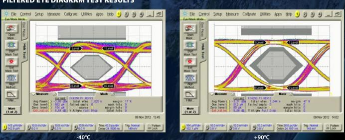
Performance of Glenair Size #8 optoelectronic contact filtered eye diagrams at 4.25Gbps demonstrates suitability of the technology for high throughput, high-bandwidth demand satellite applications including remote sensing and earth observation (climate, vegetation, forest biomass, aridity, ice caps, wind speeds, sea levels, magnetics), communication, quantum key, telecoms, and worldwide expansion of internet coverage.
