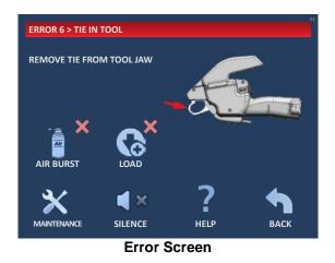
**POSSIBLE CAUSE:** This occurs if the cable tie reaches the tool but is prevented from completing the cycle. This may be due to a large air pressure drop, too large of a bundle, improper feeder hose connections, an obstruction blocking the cable tie path, pushing the front jaw in at the start of the cycle, a severe bend or twist in the feeder hose, or the tool jaws are opened during the cycle.
