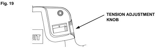
Pull the trigger to cut the tie and eject the tip from the tool. Reset the tension by turning the tension adjustment clockwise 2 clicks. If the message remains, the system will not operate. Write down the message and notify the maintenance department.
