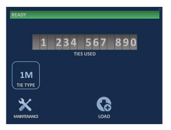
The **"Maintenance"** icon *w* will advance to the next menu level to activate the other dispenser functions. The functions are displayed as icons and have cascading functions. Press the icon to go up (forward) one
