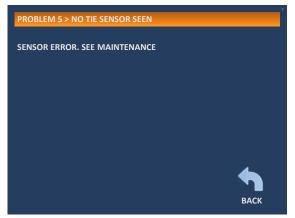
**POSSIBLE CAUSE:** A buildup of debris in the dispenser rotary caused by not cleaning the tie sensor often enough.
