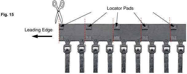
2. Pull the end of the cable tie strip and guide the cable tie carrier strip against the back edge of the ramp as the cable ties enter the cover opening. Slide the carrier strip into the opening until it stops.
