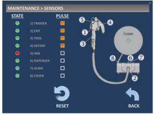
The Pulse represents the sensor events that have been triggered successfully during the last cycle. The Level represents the status of the sensors at any given time. Reset clears all triggered events of the last cycle. Pressing the **"Back"** icon after reviewing this display will return to the previous menu level.
