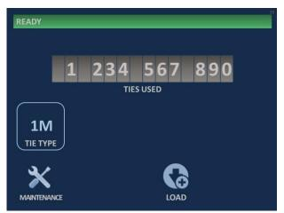
2. Press the **"Tie Type"** icon and the system will advance to the convey pressure screen to help the user set the correct internal regulator pressure per the tie type (1M or 1.5M).
