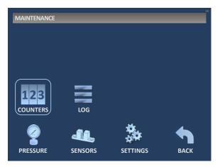
The **"Maintenance"** menu provides users with the ability to setup the system, review data and update counters. **"Back"** icon will return to the last menu level (Level 1: Ready Menu).
