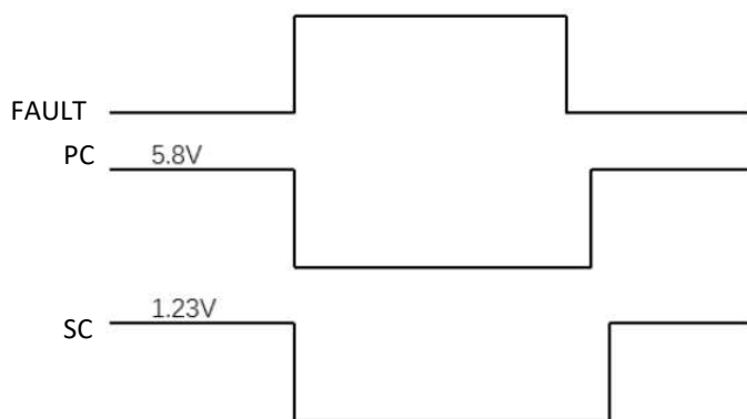
Fig.5 PC/SC module alarm timing
